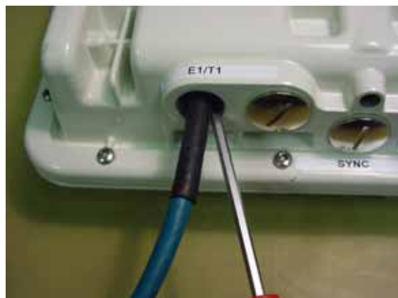
Figure 141 - Disconnecting the ODU
