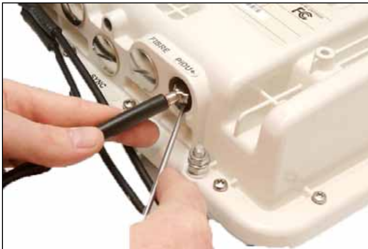
Figure 32 - Disconnecting the ODU
