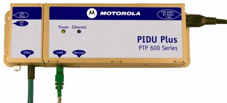
Figure 5 – PIDU Plus Recovery Switch Location
