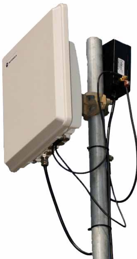
Figure 3 – PTP 600 Series Bridge Outdoor Unit (ODU)
