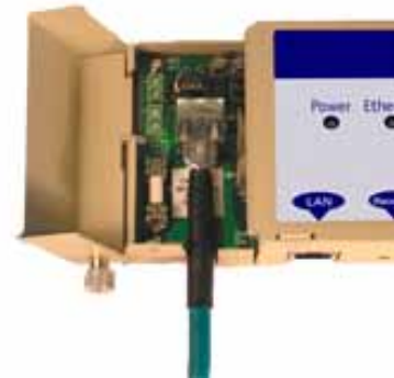
Step 2: Plug in the ODU into the PIDU Plus Cable ensuring that it snaps home
