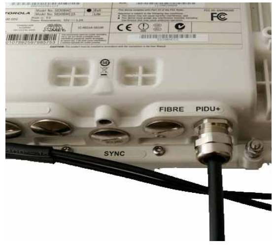
Step 4: Screw on the clamping nut and tighten
