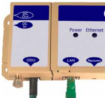
Figure 33 - Making the Network Connection at the PIDU Plus
