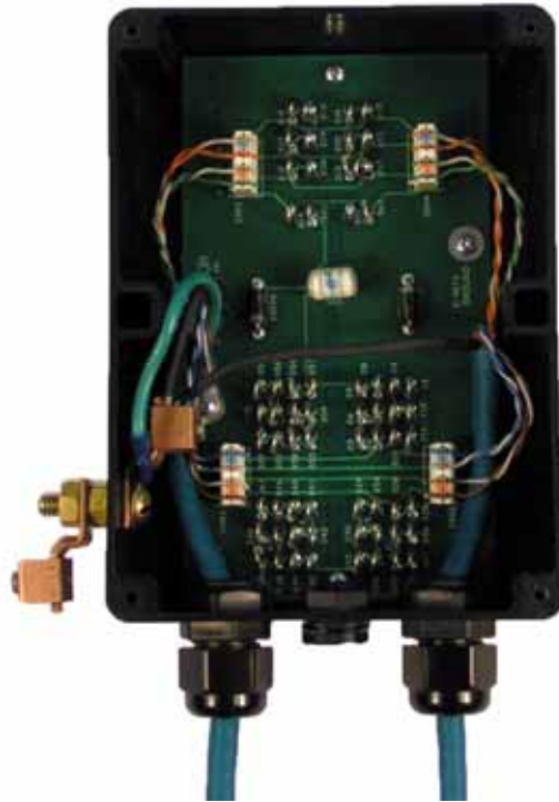
Figure 147 - Surge Arrestor ALPU-ORT Connection Illustration
