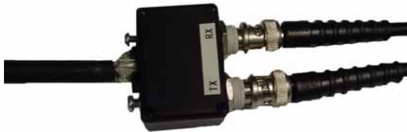
Figure 142 - Example of a Balun
